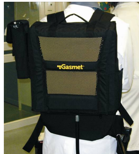
Fig. 2. Gasmeter Dx – 4030 in use at an operating room with back-pack.
